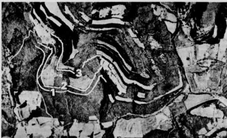
Figure 2. Aerial photograph of Hammond Mountain, southeastern Washington County. North is to left, scale is approximately 1:31,000. First, second and third sandstone units of the lower Atoka Formation form prominent bluff lines on the mountainside. All units dip to the southeast, into the Drakes Creek fault zone. U.S.D.A. (A.S.C.S.) photograph, March, 1972.
